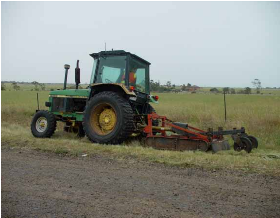
Figure 2. Roadside maintenance such as slashing can contribute to weed dispersal.
